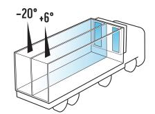
Special flexible unit with two different temperature zones.
